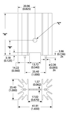
A Dim 63.50 B Dim 21.59 C Dim 3.66
